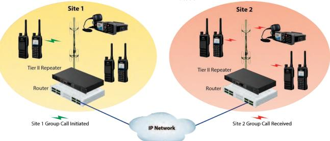
IP Connect systems can link multiple repeaters at a site and can support up to 255 locations by configuring primary and secondary repeaters. Each location can use a different frequency or DMR standard compliant radios of any manufacturer.
